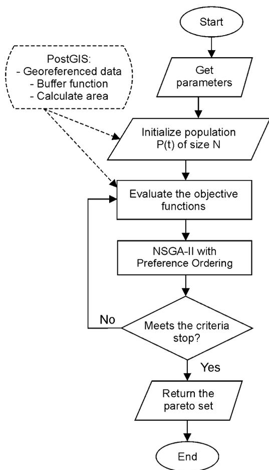
**Fig. 3** Flowchart of the computational resolution method implemented for optimal well selection. The flowchart shows the process of evaluation of each solution based on the NSGA-II algorithm
