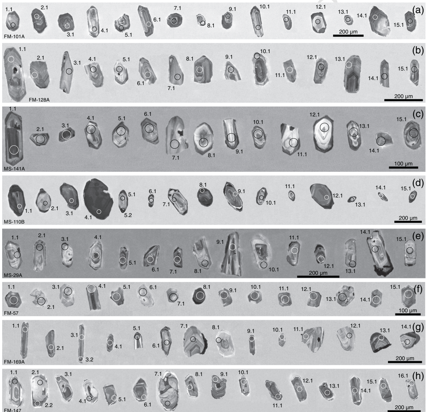
Fig. 3. Cathodoluminescence images showing the zircon grains analyzed by U–Pb SHRIMP isotopic technique. Black and white circles indicate the location of the performed spot analyses. Numbers in the bottom left corners are sample numbers discussed in the text.
